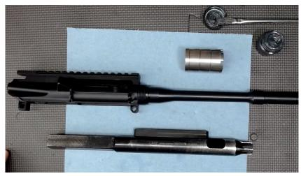
**Step 1:** With a bare barrel inserted into your upper receiver assembly, secure your upper receiver in an appropriate fixture so that sufficient torque can be applied without damage.
