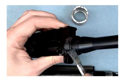
**Step 3:** Insert your 1/2" drive torque wrench into the supplied barrel nut wrench and set wrench (if required) to 60 ft/lbs.
